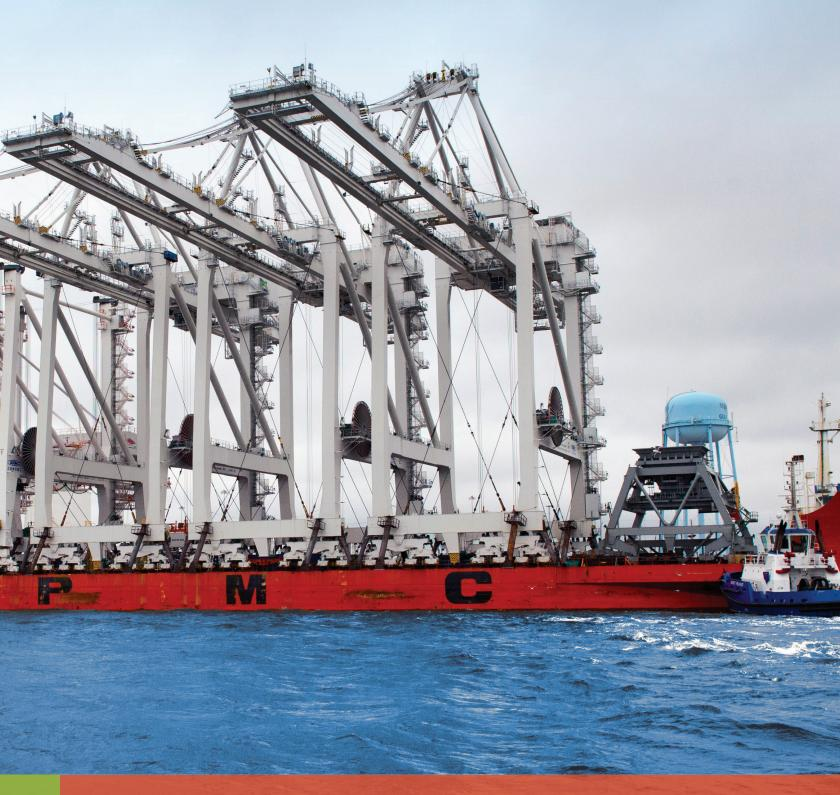
The Port of Gulfport's three new ship-to-shore gantry cranes arrived on March 18, 2016. The cranes were constructed in Shanghai, China and made a three month journey to Gulfport fully assembled.
